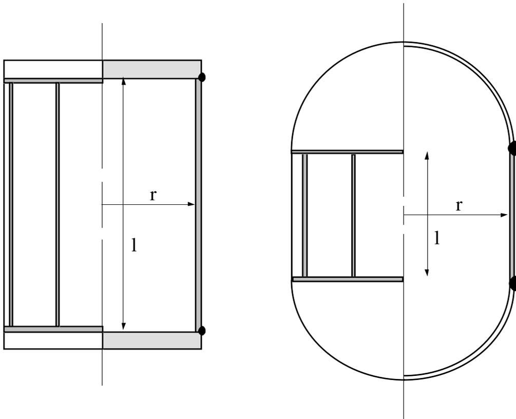
Figure 6: Hemispherical and flat head air tank designs.
