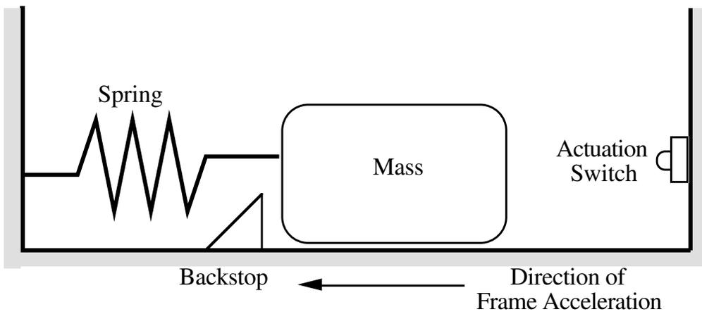
Figure 5: Example: accelerometer.
