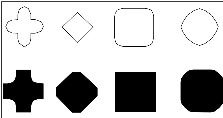
Figure 10: (A) Initial mask shapes; the squares are .8 mm across. (B) Predicted shapes derived from Figure 9. Compare with Figure 11. In both A and B, The top row of figures represents “pegs” while the bottom row represents “holes”.
