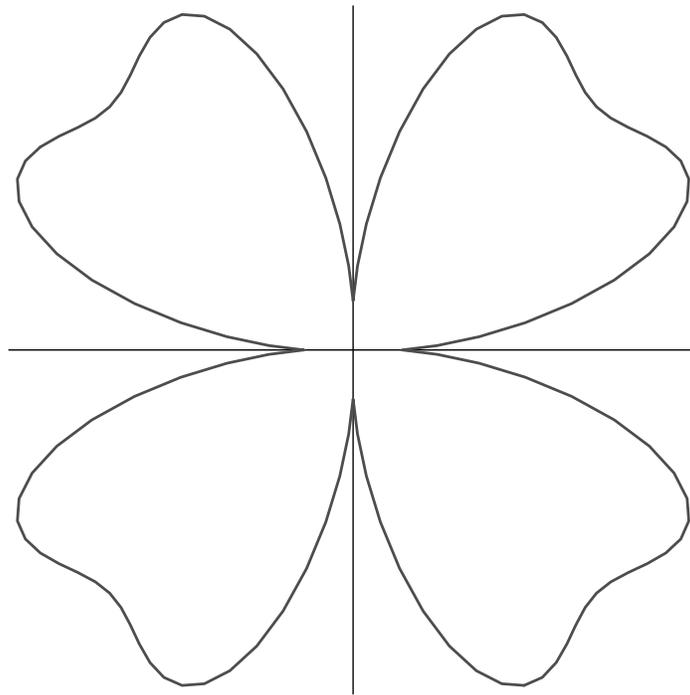
Figure 1: A qualitative example of an etch rate diagram. The formula for this rate in terms of angle  $\theta$  is given above the figure. Etchants such as KOH and EDP have (100) etch rate diagrams which are very similar to the above figure.
