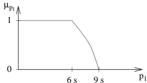
Figure 1. Imprecise functional requirement “less than 8 seconds”.
