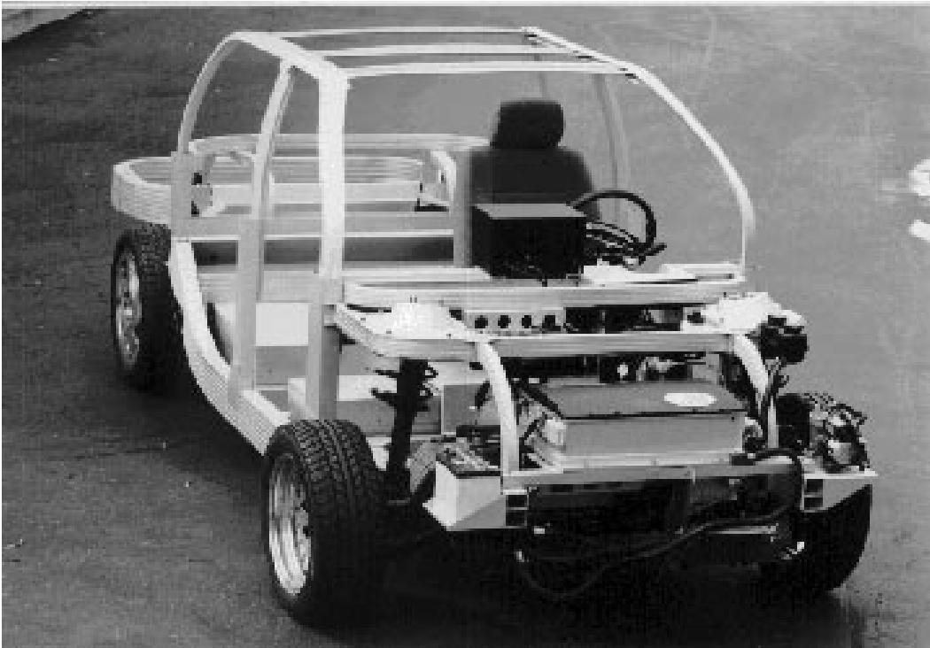
Figure 2.2 Amerigon's electric vehicle chassis © Copyright 1996 CAL-START, Inc., all rights reserved. Permission to use granted April 30, 1996.
