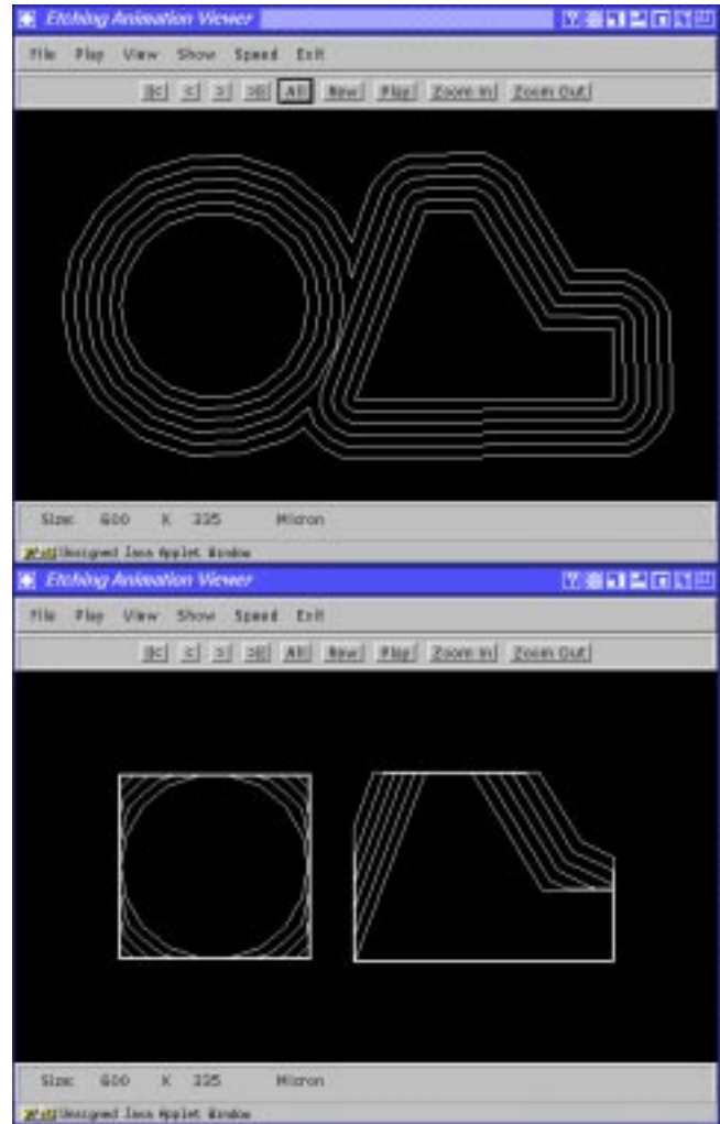
Figure 4: Animation Output Applet: (initial mask shown in Figure 3) top - isotropic etchant, bottom - anisotropic etchant. Each contour is the two dimensional shape at a different time.
