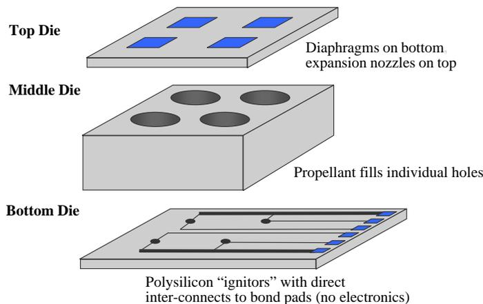
Fig. 3. Configuration of the Digital Propulsion micro-Thruster Chip.
