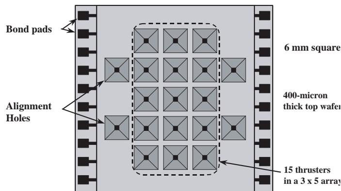
Fig. 4. Top View of the Digital Propulsion Configuration.
