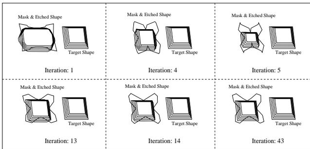
Figure 5: Evolutionary Algorithm Synthesis Result For Solid Square Target Shape.
