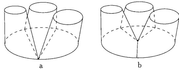
Figure 1: Comparing reconstructed surface (a) without and (b) with added vertex. *Source:* J.D. Boissonnat, Three dimensional reconstruction of complex shapes based on the delaunay triangulation. *INRIA Research Reports*, 1697, April 1992.
