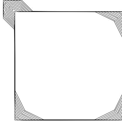
Figure 10: Simulation Results of Computed Compensation Structure, Other 3 Corners Uncompensated
